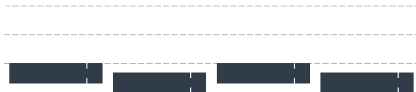
Figure 3: collocation of trucks with offsets
